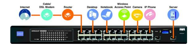
Figure 3-1: Typical Network Configuration for the SRW2024P
